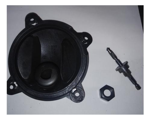
Drill a bigger hole for the centre drill bit to freely go through. Then can drill holes from backside out to front.
