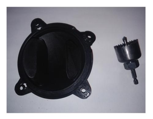
There is only 2 spots the hole saw will fit. We want a smooth hole without touching other parts of air filter lid. Since the centre bit cant be centred properly to start the hole at correct angle. Remove centre drill bit and insert saw to find.
